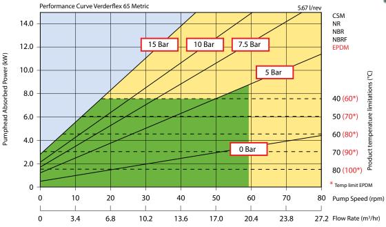
Displacement 5.67 l/revolution, Capacity is speed x 0.34 in m3/hr Minimum starting torque required: 1150 Nm Maximum peak power +20%
