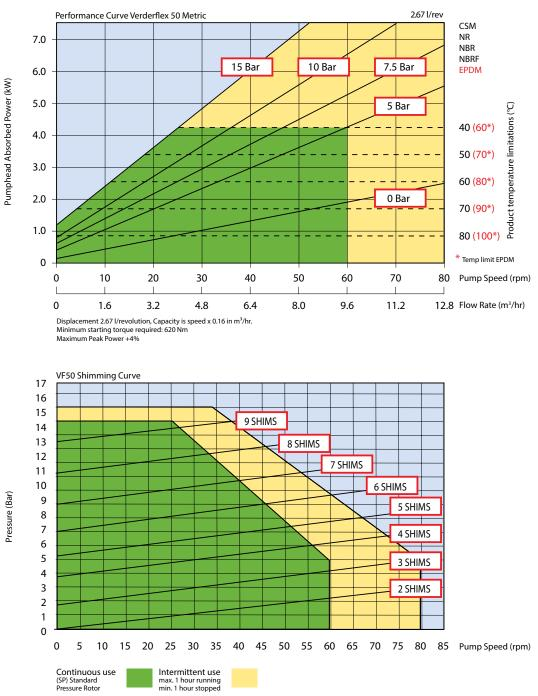
For product temperatures above 65°C and/or viscocity above 2000 mPas use one shim less than shown
