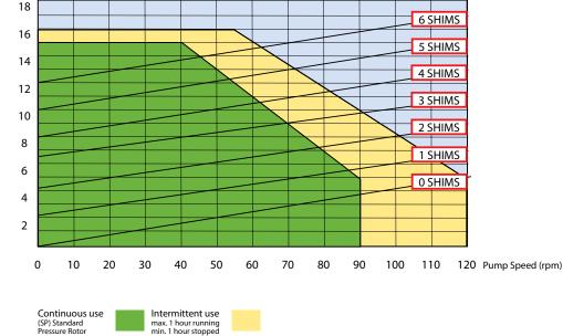
For product temperatures above 65°C and/or viscocity above 2000 mPas use one shim less than shown
