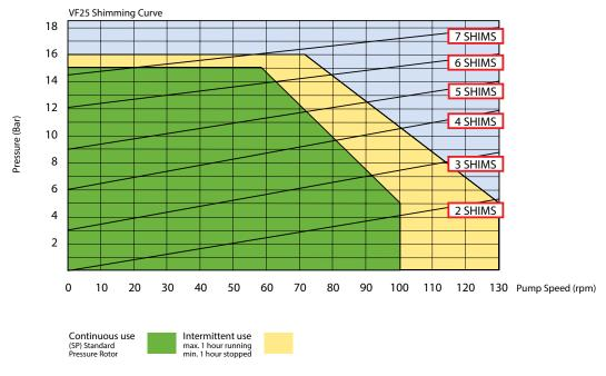
For product temperatures above  $65^{\circ}$ C and/or viscocity above 2000 mPas use one shim less than shown.
